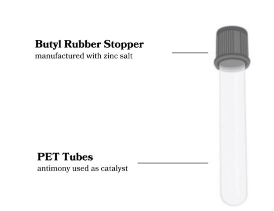
These outcomes were hypothesized to be related to the tube components: most BD stoppers consist of butyl rubber, whose manufacturing process involves the use of zinc salts, while the tubes themselves are made of polyethylene terephthalate (PET), where antimony is used as a catalyst during fabrication.
